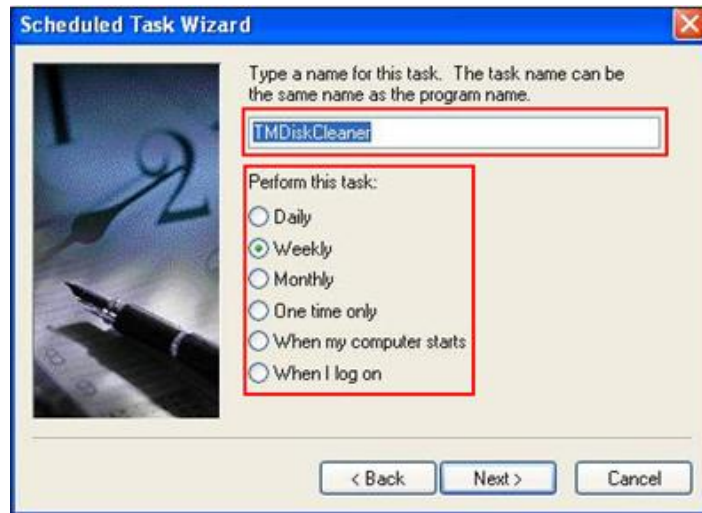
Figure 21 Scheduled task to run TmDiskCleaner tool
